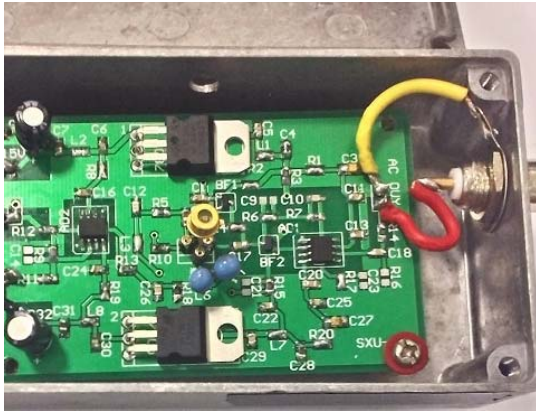
Fig. 3. Photograph of the amplifier. Many components are surface mounted (packaged in 0805), and the output connectors are all 50 \Omega -BNCs.
